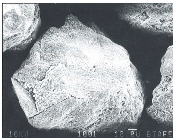
Plate 3 - Marginal impact fracture system probably from pestle. Longest Crack is 15.6 \mu m.
