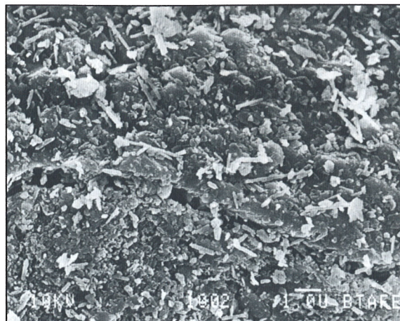
Plate 2 - Elastic brittle crack 0.5-1.0 \mu m wide. Domain change toward crack from loose, compacted, to cemented.
