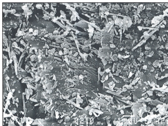
Plate 5 - Felspar cleavages exuding halloysite crystals 4 \mu m long. Crack or grain boundary on left.
